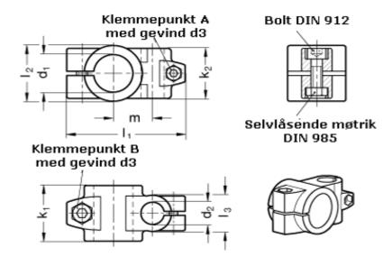
Adjustable clamp lever for d3 = GN 911-M 8-32 have to be ordred separately Adjustable clamp lever for d4 = GN 911-M 6-25 have to be ordred separately d1 = 20
